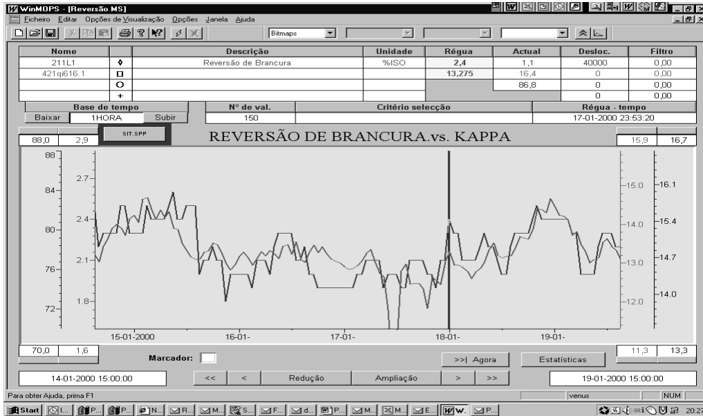
Figure 2. Variation of brightness reversion (machine sheet) with digester k number
