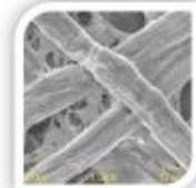
Fibres refined at 20 kWh/t SEL 0.05 Ws/m
