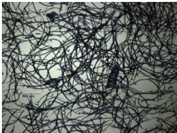
Figure 1. Eucalyptus vessel cells in pulp (hydrocyclone inject, Noss)
