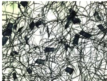
Figure 2. Eucalyptus vessel cells in hydrocyclone reject (Noss)
