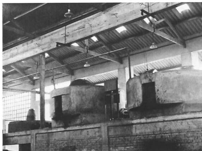
In the rotary pulp grinders, through the pressure and friction of the rotating grinding wheels, the raw material was broken down to form small uniform particles. Rotary pulp grinders installed in mill of Adamas do Brasil S.A., Osasco, SP, 1956
