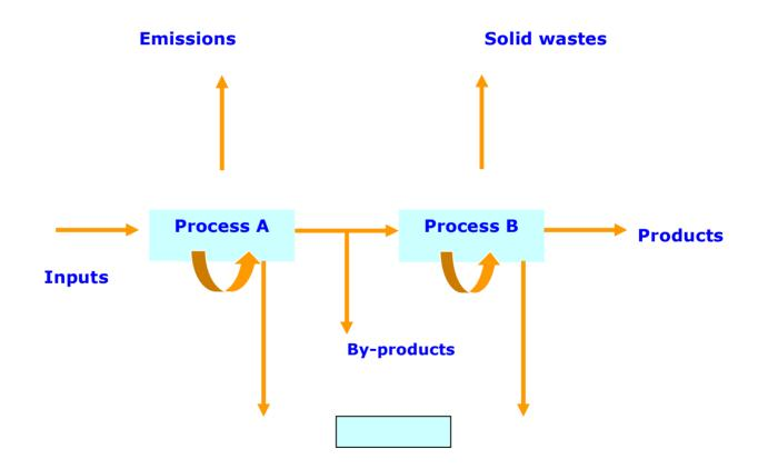
Working out mass flow and energy transfer and utilization balances belongs to the strategies to minimize or to eliminate the losses and to find the inefficiencies. A material or mass flow balance consists in fact in following the way the materials (elements, compounds, substances) run along the production process. They may be done either in a wide scope, involving control units or with a scope as wide as the whole mill, or an area of the company.
