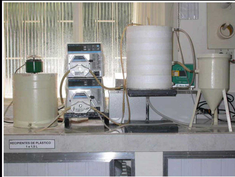
Aerobic membrane bioreactor
